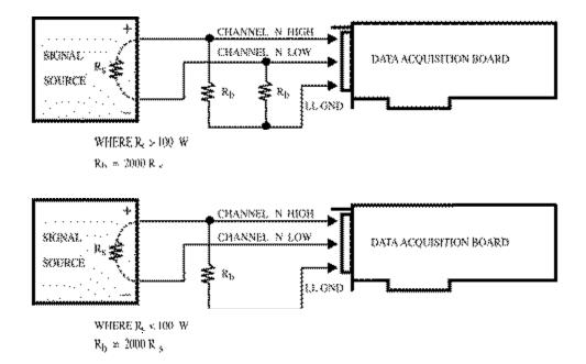
Figure 3. Differential input schemes for DAQ cards.
